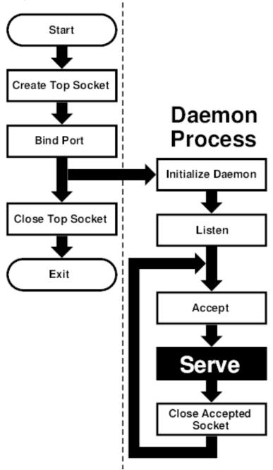
This flowchart is good for *sequential servers*, i.e., servers that can serve one client at a time, just as we were able to with our *daytime* server. This is only possible whenever there is no real "conversation" going on between the client and the server: As soon as the server detects a connection to the client, it sends out some data and closes the connection. The entire operation may take nanoseconds, and it is finished.
