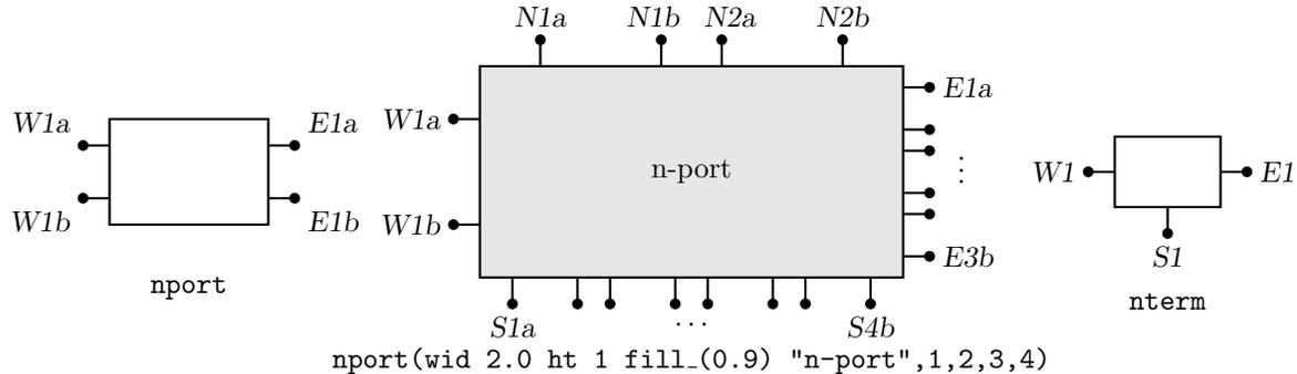
**Figure 26:** The `nport` macro draws a sequence of pairs of named pins on each side of a box. The pin names are shown. The default is a twoport. The `nterm` macro draws single pins instead of pin pairs.
