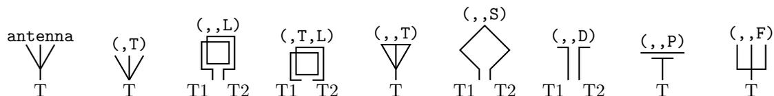
**Figure 21:** Antenna symbols, with macro arguments shown above and terminal names below.
