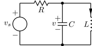
**Figure 2:** The file `quick.m4` and resulting diagram. There are several ways of drawing the same picture; for example, nodes (such as `Origin`) can be defined and circuit branches drawn between them; or absolute coordinates can be used (e.g., `source(up_ from (0,0) to (0,0.75))`). Element sizes and styles can be varied as described in later sections.
