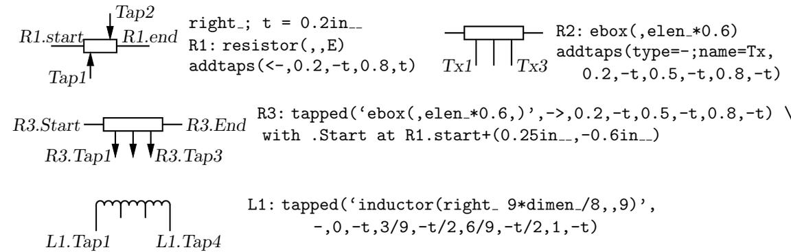
**Figure 18:** Macros for adding taps to two-terminal elements.
