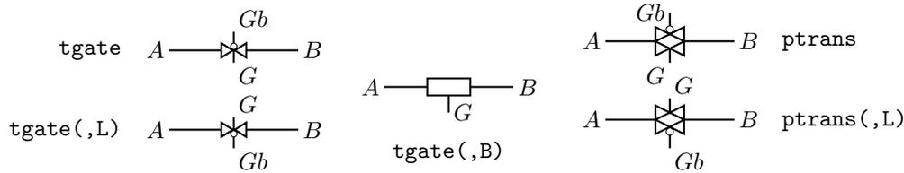
Figure 41: The `tgate`(*linespec*, [*B*] [*R*|*L*]) element, derived from a customized diode and `ebox`, and the `ptrans`(*linespec*, [*R*|*L*]) macro. These are not two-terminal elements, so the *linespec* argument defines the direction and length of the line from *A* to *B* but not the element position.
