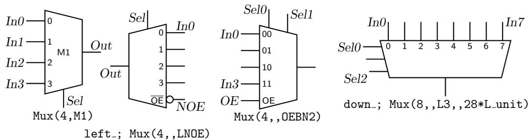
Figure 50: The `Mux(input count, label, [L] [B|H] [N[n] |S[n]] [[N]OE], wid,ht)` macro.
