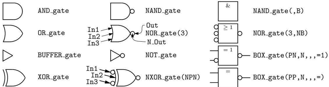
Figure 46: Basic logic gates. The input and output locations of a three-input NOR gate are shown. Inputs are negated by including an `N` in the second argument letter sequence. A `B` in the second argument produces a box shape as shown in the rightmost column, where the second example has AND functionality and the bottom two are examples of exclusive OR functions.
