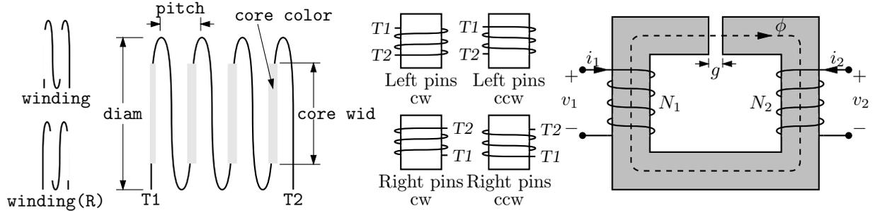
Figure 28: The `winding(L|R, diam, pitch, turns, core wid, core color)` macro draws a coil with axis along the current drawing direction. Terminals T1 and T2 are defined. Setting the first argument to R draws a right-hand winding.
