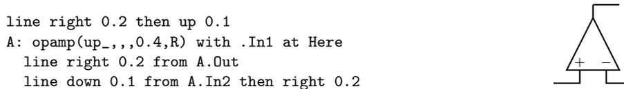
Figure 23: A code fragment invoking the `opamp(linespec,-,+,size,[R][P])` macro.
