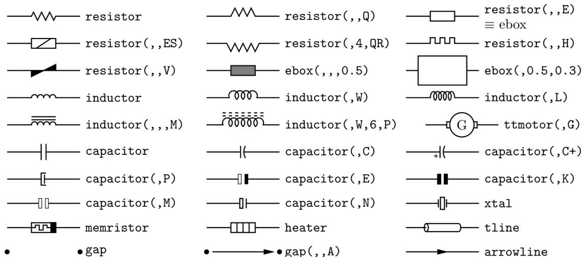
**Figure 7:** Basic two-terminal elements, showing some variations.
