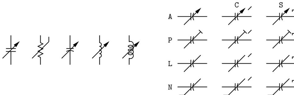
**Figure 13:** Illustrating `variable('element',[A|P|L|[u]N][C|S],angle,length)`. For example, `variable('capacitor(down_ dimen_))` draws the leftmost capacitor shown above, and `variable('resistor(down_ dimen_)',uN)` draws the resistor. The default angle is  $45^\circ$ , regardless of the direction of the element. The array on the right shows the effect of the second argument.
