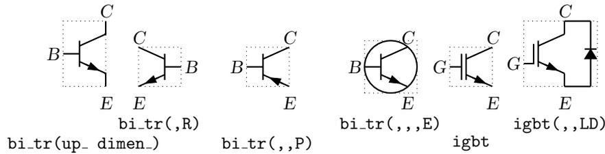
Figure 35: Bipolar transistor variants (current direction upward).
