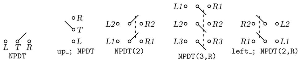
Figure 30: Multipole double-throw switches drawn by `NPDT(npoles, [R])`.
