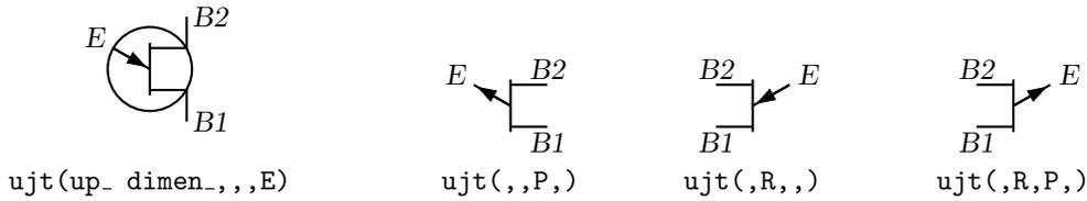
Figure 39: UJT devices, with current drawing direction up.
