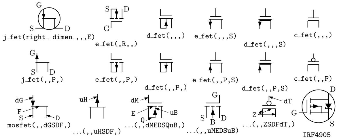
**Figure 42:** JFET, insulated-gate enhancement and depletion MOSFETs, and simplified versions. These macros are wrappers that invoke the `mosfet` macro as shown in the bottom row. The two lower-right examples show custom devices, the first defined by omitting the substrate connection, and the second defined using a wrapper macro.
