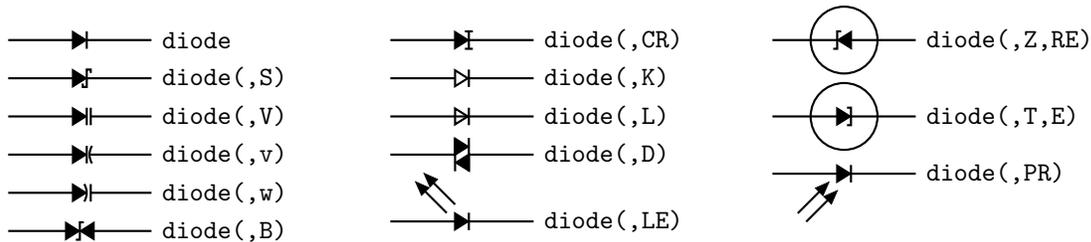
Figure 9: The macro `diode(linespec,B|CR|D|K|L|LE[R]|P[R]|S|T|V|v|w|Z,[R][E])`.
